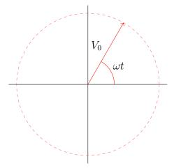
At any given time, the projection of this phasor vector onto the real axis gives the actual physical voltage being driven into the circuit.
