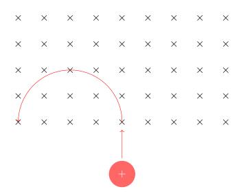
The direction in which the particle deflects can be found using the right hand rule for cross products.
