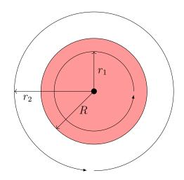
For an Amperian loop taken inside of the cylinder, we are only enclosing some section of current.
