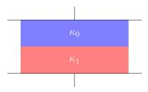
we can think about this as a system of two capacitors in series, with one of each containing each of the different dielectrics. The equivalent dielectric constant, then, is
