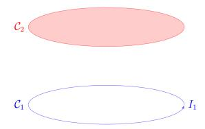
The current  $I_1$  in  $C_1$  induces a magnetic field that pierces the area enclosed by  $C_2$ , thus creating magnetic flux through  $C_2$  which is directly proportional to  $I_1$ . We define a quantity called the *mutual inductance* from  $C_1$  to  $C_2$ :
