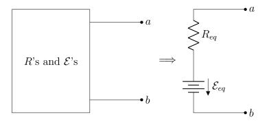
Often times, we are trying to analyze the current through some load  $R_L$ or other complex circuit (for example, one involving a capacitor) to the two outgoing terminals of the blackboxed circuit (i.e. we are trying to find the Thevenin equivalent current  $I_{eq}$  between terminals *a* and *b*). To do this, we need to first find  $\mathcal{E}_{eq}$  and  $R_{eq}$ , and then calculate
