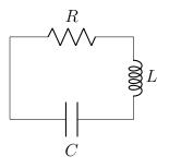
Extending the analogy to a simple harmonic oscillator, the resistor in this circuit acts as a kind of dashpot, adding a damping factor to the differential equation.
