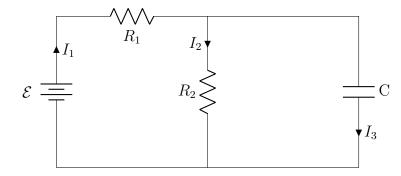
When solving, we should keep in mind two limiting conditions. At t = 0, the capacitor, initially uncharged, will function effectively as just a wire; therefore, all of the current will try to flow through that second branch, and momentarily,
