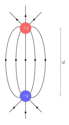
At any point, the electric field is the sum of the electric field contributions from the positive charge  $\mathbf{E}_+$  and the negative charge  $\mathbf{E}_-$ . Given that the dipole is centered at the origin and extends along the z axis, we have the following expression for the total field:
