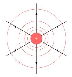
The red lines indicate the equipotential lines around this point charge. Notice that these equipotentials are orthogonal to the electric field lines. Recall that the level curves of a multivariable function are normal to its gradient. This leads us into another important idea about the electric potential:
