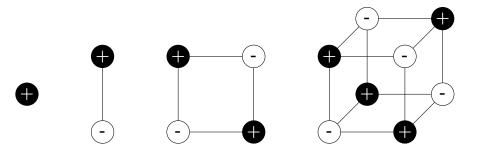
Additionally, the lowest non-zero moment of a charge distribution is an indication towards how the strength of a field varies based on distance. Dipoles have no net monopole moment, so the highest-order surviving term is on the order of  $r^{-3}$ . Extending this further, charge configurations that have a quadrupole moment but have no net dipole moment or monopole moment will generate a field that falls on the order of  $r^{-4}$ .
