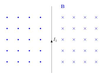
where the blue markings represent the field going into and out of the page. Another given wire to the right of the wire in the diagram will, by the right hand rule, experience a force directed *left* if its current is going in the same upwards direction, or it will experience a force directed *right* if its current is going in the opposite direction.
