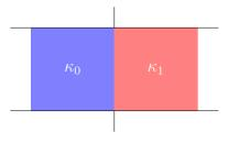
We can treat this as a system of two capacitors in parallel, yielding an equivalent dielectric constant of
